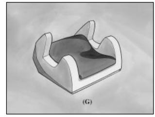
A booster seat (F, G) is designed for children who are about 40 to 60 lbs., or even up to 80 lbs. (18 to 27 kg, or even up to 36 kg), and about four to eight years of age. A booster seat is designed to improve the fit of the vehicle's safety belt system. Booster seats with shields use lap-only belts; however, booster seats without shields use lap-shoulder belts. Booster seats can also help a child to see out the window.
